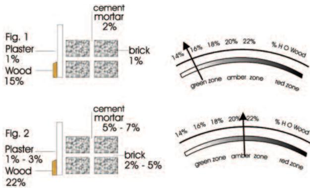
This diagram illustrates the different moisture contents of different building materials, all in moisture equilibrium. The upper example shows the air-dry (safe) condition; the lower example a wet (dangerous) condition. The figures on the right are WME readings on a Protimeter moisture meter.
