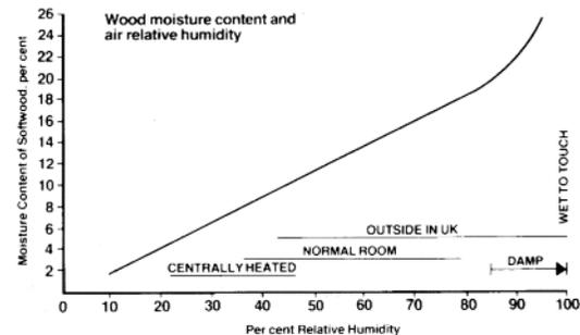
The graph shows the approximate relationship between the relative humidity (r.h) of air and the moisture content of typical softwoods. The horizontal lines show the typical range of humidities met in various circumstances. Wood kept in these environments will gradually come into equilibrium at the moisture content levels indicated on the vertical scale. 75% rh. is 'safe' in building materials.
