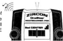
In cases of deeper studs (or thicker walls) two bars will show on the Signal Strength Indicator and only the SpotLite and four middle bars will illuminate. If you still can't locate a stud, try the next step.
