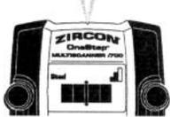
Quickly (within one second) release and re-press the handle down. The scanner will enter the **High Sensitivity Mode** and the Stud Scan Mode Indication will flash continuously. The centre of a very deep stud will be indicated by the four middle bars illuminating.
