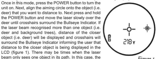
TIP: While pressing the POWER button, you can move the device slowly from object to object and intentionally force the laser to hit multiple objects to ensure that you are only displaying the closest of the objects recognised by the laser.
