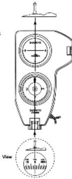
Fig. 5. The hairline is seen against the target
