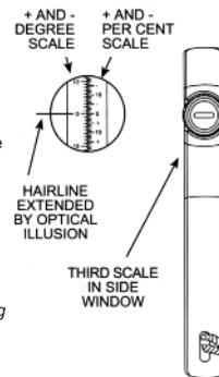
horizontal plane at eye level. The right-hand scale gives the height of the point of sight from the same horizontal eye level, and it is expressed in percent of the horizontal distance. The following example illustrates the procedure.
