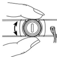
Fig. 1. Adjusting optics
