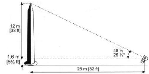
Fig. 8. Measuring height of a pillar
