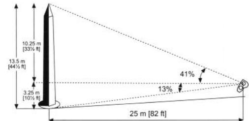
Fig. 9. Taking two readings
