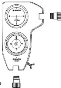
Fig. 2. Removing the eyepiece
