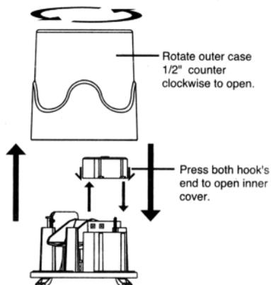
2. Remove the tape from the bucket inside so it moves freely.
